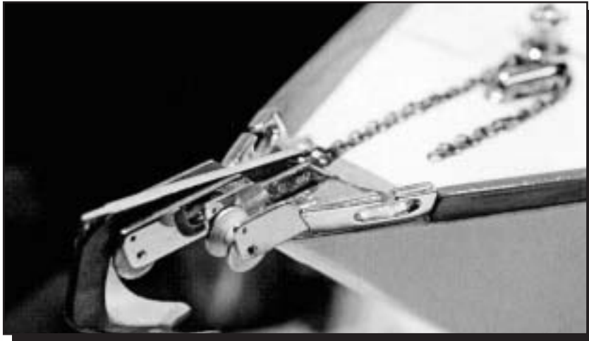
PRECIOUS: Melting gold in a crucible, Eddy then casts fittings such as this pulpit and anchor.
