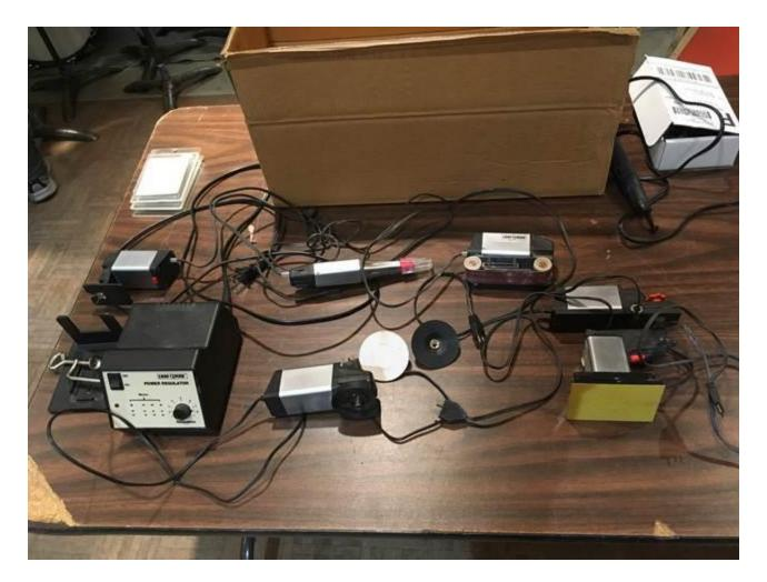
Starting upper left and clockwise: Jig saw with accessory table mount, pencil sander, belt sander, jointer, oscillating sander, disc sander/grinder, voltage regulator.
