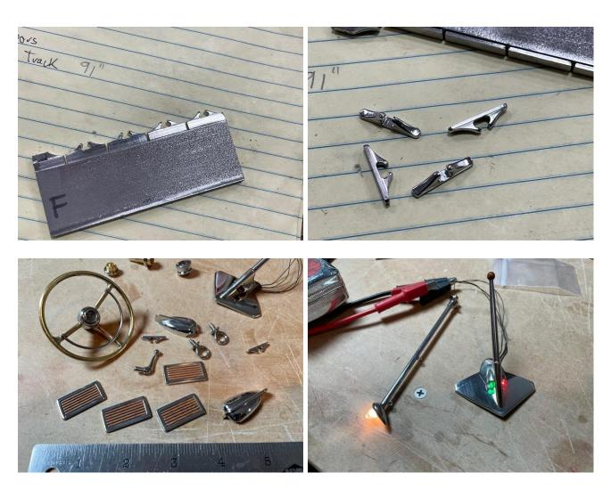
Several different types of metal were utilized for the various parts. In addition to the creation of parts is the fabrication of flags on fabric:
