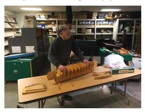
Mike explained that he always wanted to build a full size canoe from scratch and did the model version as a warm up. Based on plans from Ted Moores, Bear Mountain Boats, Mike adjusted scale on a copy machine for the various sized forms in the photo. The canoe was actually completed about a year ago. Here is the finished boat:
