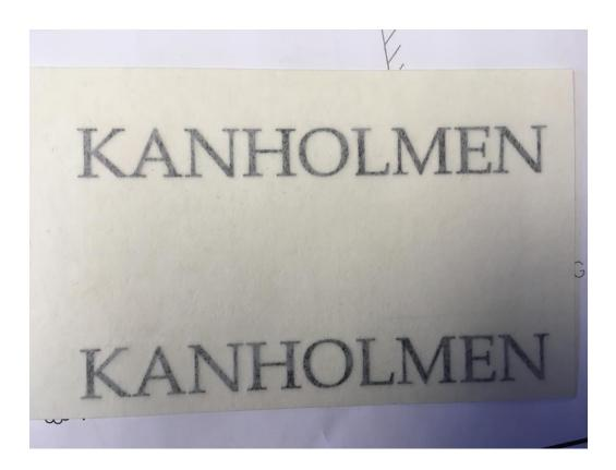
The lettering can then be lifted off the carrier paper and pressed onto the desired surface. What we discovered was that the text for "STOCKHOLM" in Book Antiqua non-bold was cut out with the line work so fine (see photo previous) that it was difficult to peal the excess material away without disturbing the letters, and is a demonstration of how accurately this machine can "print".
