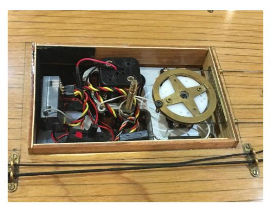
Tight access to the winch for the sails, the drum is below the wiring lower left in the opening. The wheel/pulley at the right is for the rudder.
