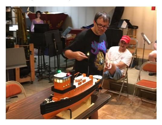
Looks a lot like a Brooklyn I think. A 12 volt system where the water that comes from the fire nozzle also cools the motor, it runs all the time. He has also fitted it with twin floating mesh bags to clean debris from the surface of the pond:
