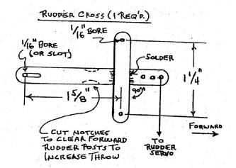
the chrome plating from the wheel collars or the solder will not adhere). The cross is also cut from 1/16" brass. I Like to drill a small hole through the top of each rudder shaft and inset a piece of soft wire. In the event that the rudder set screw loosens, the rudder can not drop out and end up on the bottom of the lake.
